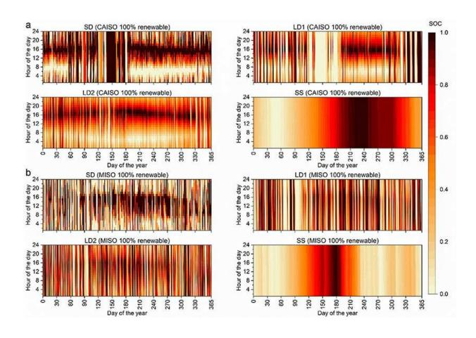
Normalized state of charge (SOC) for short-duration (SD), long-duration (LD1 and LD2), and seasonal storage (SS) in CAISO and MISO. (a) Normalized SOC for devices on CAISO with 100% renewable energy mix. (b) Normalized SOC for devices on MISO with 100% renewable energy mix. SOC = 1 (dark red) implies that the storage device is full. SOC = 0 (light red) implies that the storage device is empty. Credit: National Renewable Energy Laboratory
