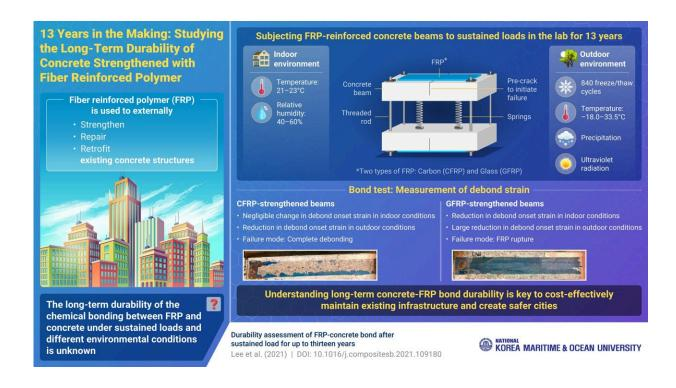
Fiber reinforced polymer coatings are an affordable way to externally strengthen concrete structures, but how long does the protection last? Scientists find out. Credit: Korea Maritime and Ocean University
