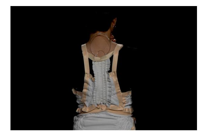
As an initial test application of the material, the team made a type of undergarment that singers can wear to monitor and play back the movement of respiratory muscles, to later provide kinesthetic feedback through the same
