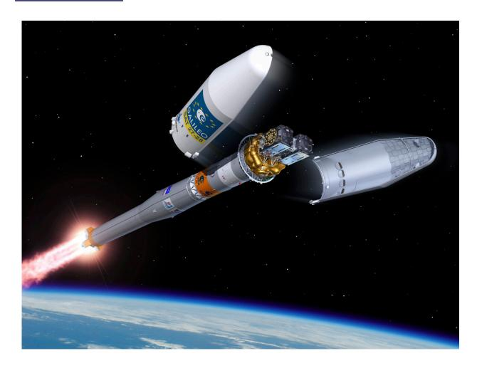
Galileos 27-28 pictured during their ascent to orbit on their Soyuz launcher. The satellites are protected by a launch fairing, but once the Soyuz has passed through the atmosphere, this fairing can then be ejected. Credit: ESA P. Carril
