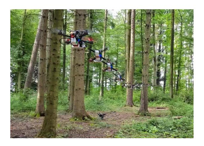
The autonomous drone navigates independently through the forest at 40 km/h. Credit: UZH
