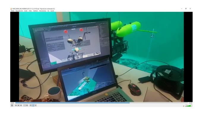
A research team from the Interactive and Robotic Systems Laboratory at the Universitat Jaume I in Castelló has developed software that allows underwater robots with manipulation capabilities to be controlled remotely in a more efficient way, as it offers a computer graphic interface and prior realistic simulation. The new technology amends, in the context of underwater scenarios, the lack of simulation systems and
