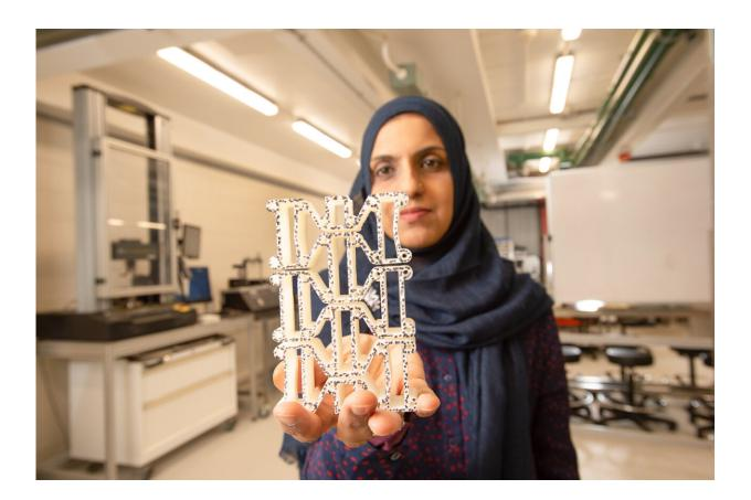
Dr Tatheer Zahra was inspired by a material used in running shoes and memory foam pillows to design a 3D-printed product that could help protect buildings from collision damage and other high impact forces, equivalent to a car traveling at 60km/hr. Credit: QUT
