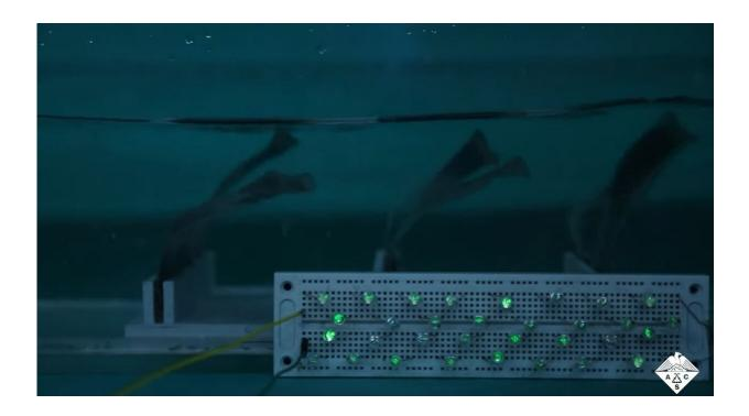
A flexible triboelectric nanogenerator (TENG) mimics the way seaweed sways to efficiently convert ocean waves into electricity. Credit: American Chemical Society.
