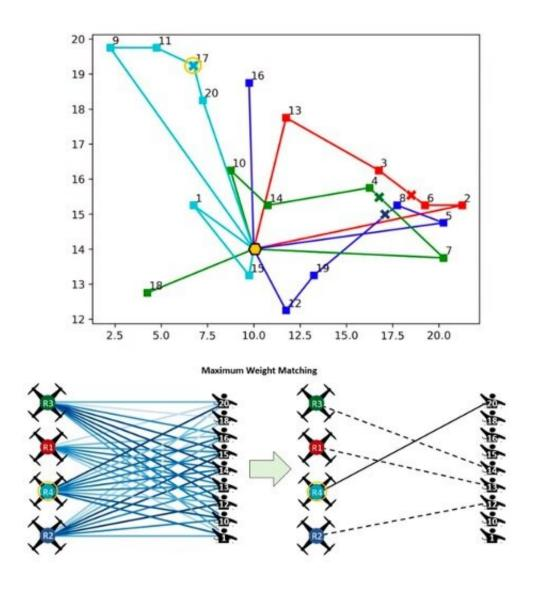
Multi-robot task allocation for a 4-robot team performing a set of ~20 tasks – The top diagram shows the routes traced by 4 robots as they visited different tasks, as decided by simulated execution of our algorithm by each robot; each robot starts and ends at the same depot, marked by the yellow hexagon. The
