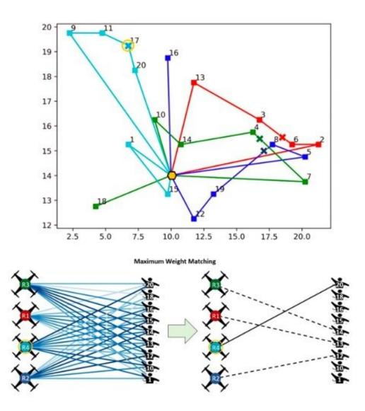
Multi-robot task allocation for a 4-robot team performing a set of  $\sim 20$  tasks – The top diagram shows the routes traced by 4 robots as they visited different tasks, as decided by simulated execution of our algorithm by each robot; each robot starts and ends at the same depot, marked by the yellow hexagon. The
