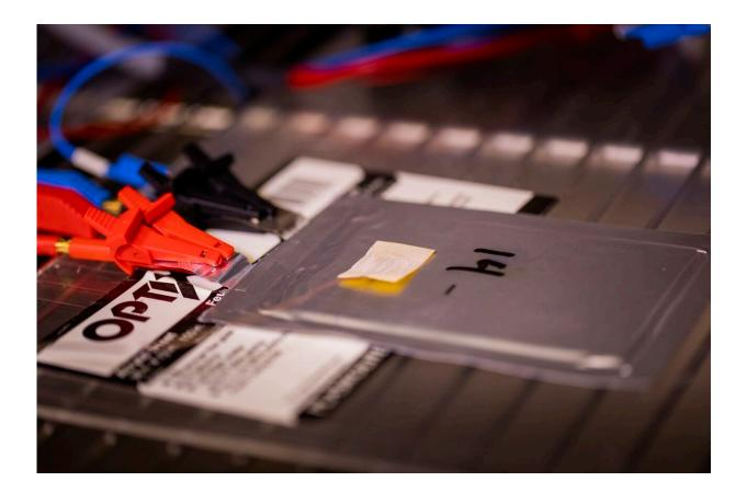
Prototype lithium-ion batteries built at the University of Michigan Battery Lab undergo diagnostic measurements inside an environmentally controlled chamber. Credit: University of Michigan
