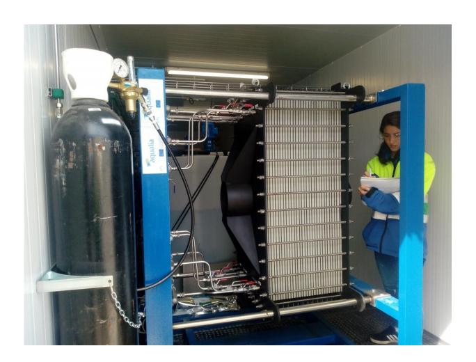
Electro-active bacteria desalinate and sterilise water making it suitable and safe. Credit: © FCC AQUALIA SA
