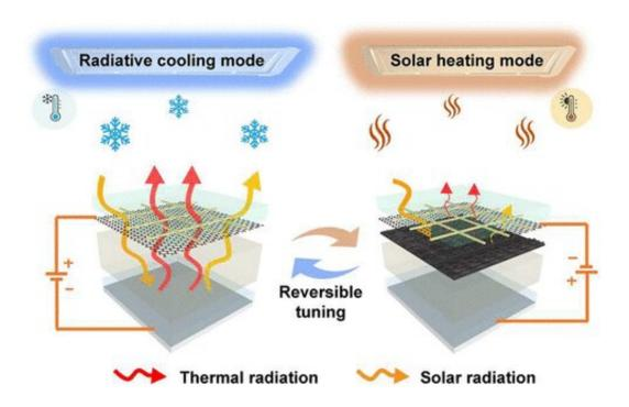
An exploded look at the layers of a new passive heating and cooling technology that is tuned to interact with both visible light and thermal radiation. Credit: Po-Chun Hsu, Duke University
