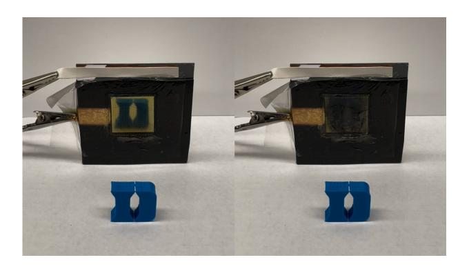
A demonstration of the "smart-window-like" portion of the passive heating and cooling technology. Electricity causes the device to either clear (left) to reveal a mirror that reflects sunlight and allows heat to escape, or to darken with tiny nanoparticles (right), which traps both sunlight and heat. Credit: Po-Chun Hsu, Duke University
