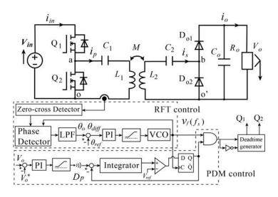
Figure 3: Diagram of the main circuit and controller in the newly developed wireless power transfer system. Credit: Kobe University
