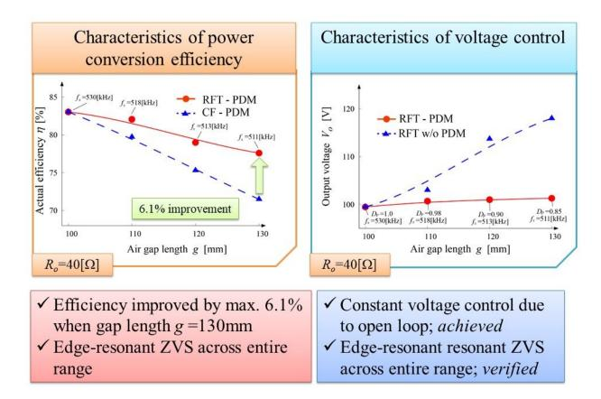
Figure 4: Comparison with existing technology (actual efficiency). Credit: Kobe University
