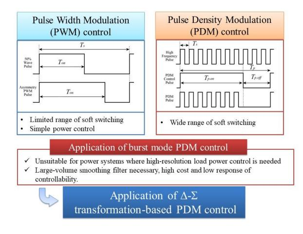
Figure 2: Technical issues with the existing technology and the solutions proposed by the new technology. Credit: Kobe University
