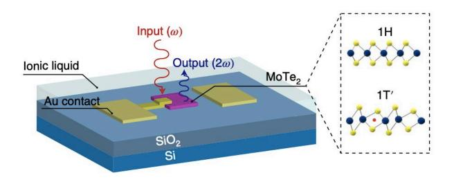
Figure summarizing the functioning of an SHG modulator. Credit: Wang et al.
