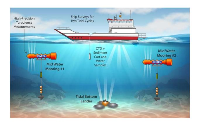
Midwater moorings and the Tidal Bottom Lander–a heavy, low-profile frame with an instrument-packed, pop-up buoy in the center–were in the water throughout July and August 2021.The ship's surveys conducted in late August measured the cross-channel variability of current speeds, sediment concentrations, salinity, and temperature. All hardware, including anchors, were designed to be recovered from the site. Credit: Al Hicks, NREL
