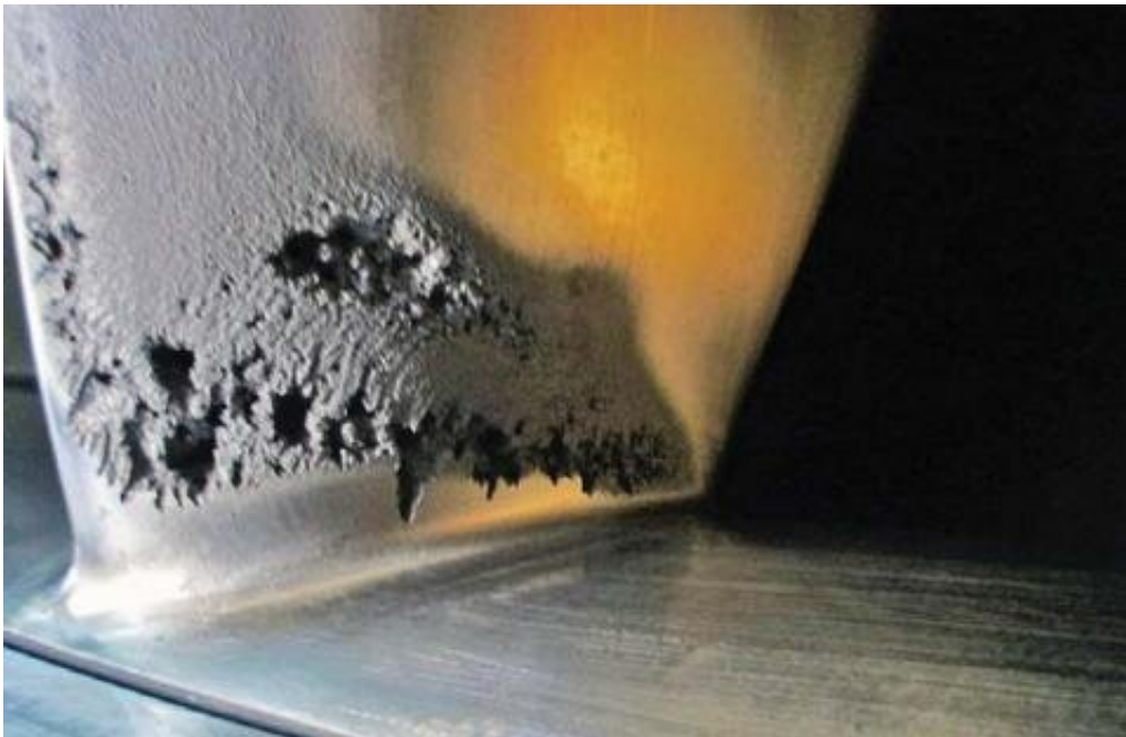
Cavitation damage to a turbine blade runner of J.R. Carr Unit 2, Feb. 2013. Credit: John Germann | U.S. Bureau of Reclamation
