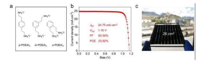
Fig. 1 a The structures of the  $PDEAI_2$  isomers. b J-V characteristics of the champion device with o-PDEAI<sub>2</sub>. c Photograph of the fabricated perovskite solar module. Credit: MK Nazeeruddin
