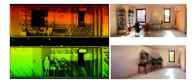
Figure 1: 3D point clouds and their respective indoor locations. Credit: University of Twente
