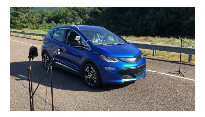
In the U.S., regulations require vehicle sounds to be detectable at certain distances for various speeds, and researchers have tested how well people detect electric vehicle sounds in terms of these requirements. Participants in the study were seated adjacent to a lane of the test facility and pressed a button upon hearing an approaching electric vehicle. Credit: Michael Roan and Luke Neurauter
