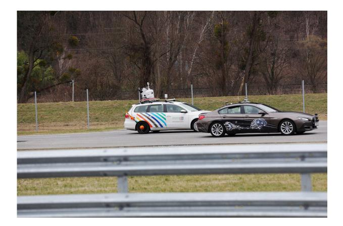
During test drives, research vehicles with very precise surveying systems create the virtual test environment. Credit: J.J. Kucek - TU Graz
