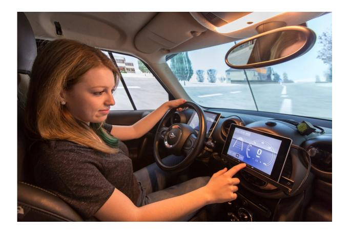
The driving simulator is an in-house development with a focus on development and testing of human-machine interfaces in the vehicle. It forms an important basis in the development process of driver assistance systems and automated driving functions. Credit: Lunghammer – TU Graz
