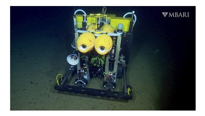
MBARI's Benthic Rover II travels across the muddy seafloor, taking photographs and measuring how much oxygen bottom-dwelling animals and microbes are using over time. The information gathered by this autonomous rover has helped scientists understand how carbon cycles from the surface to the seafloor. Credit: © 2016 MBARI
