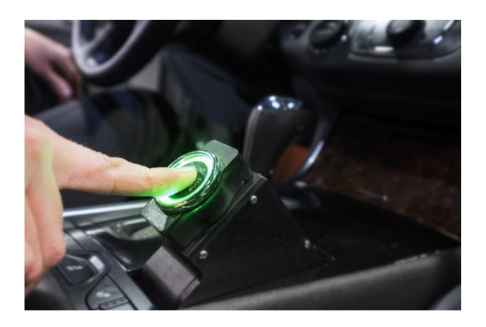
This photo, a handout by the Automotive Coalition for Traffic Safety (ACTS), shows the prototype for a touch-based system to measure alcohol in a driver's tissue, part of a system soon to be required for new cars in the United States.
