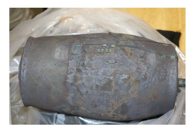
A test container after being heated to 2000 degrees Fahrenheit for four hours at Sandia National Laboratories. While the container did swell, it did not split open. The team conducted additional leak testing to determine locations of pin hole leaks. Credit: Sandia National Laboratories
