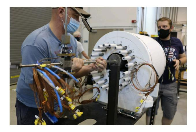
Sandia National Laboratories test engineer Austin Baird, left, and thermal test technologist Shane Adee carefully insert the test container into the custom-built heater. Each container had 18 temperature sensors and two pressure sensors. Credit: Sandia National Laboratories
