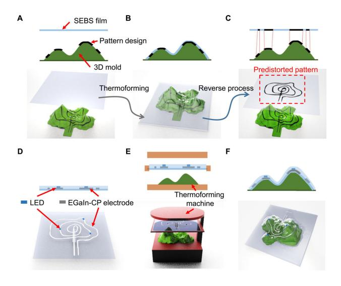
Fabrication process of the PGT3DE. (A) Design of 3DE circuit pattern on 3D mold. (B) Thermoforming simulation. (C) Predistorted pattern generation. (D) Patterning the EGaIn-CP electrode and mounting electronic devices on 2D planar SEBS film based on the predistorted pattern. (E) Thermoforming process. (F) Fabricated 3DE. Credit: *Science Advances*, 10.1126/sciadv.abj0694
