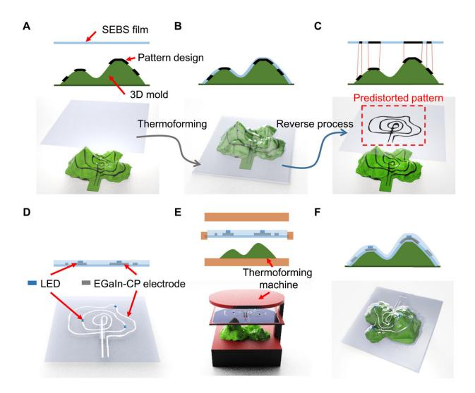
Fabrication process of the PGT3DE. (A) Design of 3DE circuit pattern on 3D mold. (B) Thermoforming simulation. (C) Predistorted pattern generation. (D)
