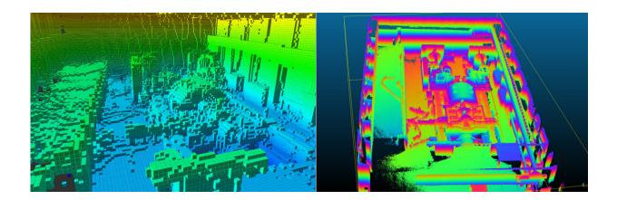
SwRI engineers used LIDAR point cloud data to reconstruct a high-resolution image of a facility that houses electric turbines at the nuclear power plant. 3D cubes, or voxels, on the left provide spatial information on the turbine facility. Several voxel images were used to create the high-resolution image of turbines on the right. SwRI specializes in data visualizations to identify damage and potential hazards following accidents at nuclear power plants and other
