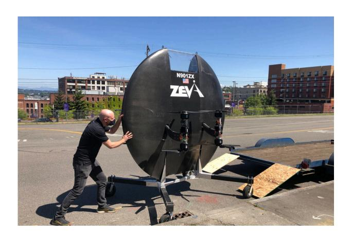
Prototype of Zeva's electrical vertical takeoff and landing (eVTOL) aircraft. Credit: Voiland College of Engineering and Architecture
