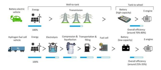
Comparison of losses across each step of the chain for battery electric and hydrogen fuel cell electric vehicle technologies. Credit: <u>CC BY-ND 4.0</u>
