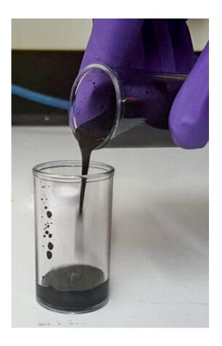
MIT researchers have developed a novel semisolid flow battery that uses a mixture containing dispersed manganese dioxide particles, along with an electrically conductive additive called carbon black, that enables efficient electrochemical energy conversion when reacted with a zinc suspension or plate. Credit: Thaneer Narayanan
