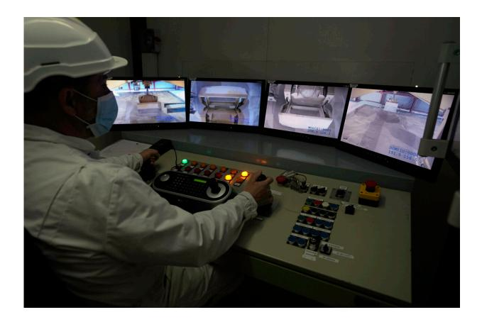
A technician pilots robots for radioactive waste storage in a concrete-sealed warehouse in the Aube region of eastern France in Soulaines-Dhuys, Friday, Oct. 29, 2021. The site holds low- to mid-level radioactive waste from French nuclear plants as well as research and medical facilities, and its concrete-sealed warehouses are designed to store the waste for at least 300 years. Credit: AP Photo/Francois Mori
