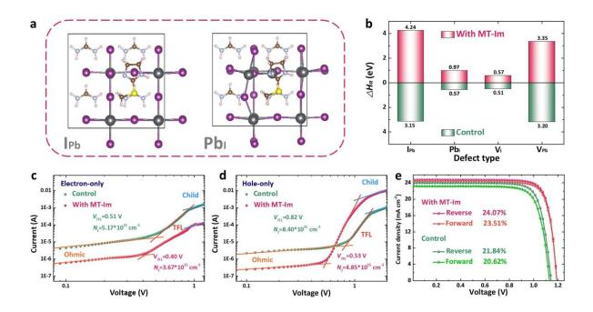
a. Theoretical calculation model; b. the formation energy ( $\triangle H\alpha$ ) of interface defects; c,d. Defect density calculation and photovoltaic performance test of perovskite solar cells. Credit: Liu Guozhen.
