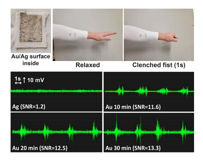
In this graphic, a compression sleeve is turned into a biosensor that measures electrical impulses generated from muscle movement. Shown is the measurement of electrical activity picked up by the sleeve when a fist is made. Credit: Huanan Zhang/University of Utah
