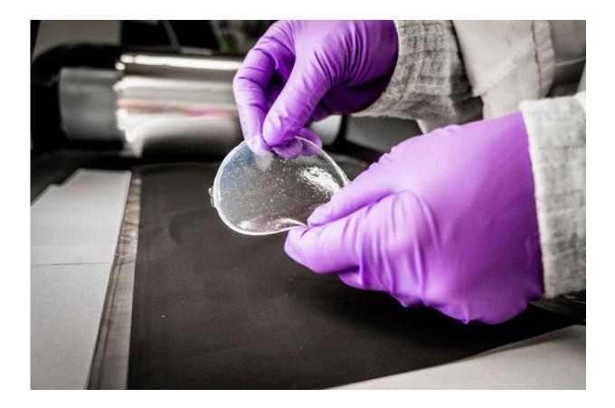
The electrolyte here is seen in the form of a gel, while the black base is a largearea lignin electrode coated on a metal collector. Credit: Thor Balkhed
