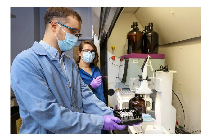
Jansone-Popova, right, uses an automated chromatography system to purify diglycolamide—an extractant used for rare-earth element separation. Popovs prepares samples for the analysis using a pipetting robot. Credit: Genevieve Martin/ORNL, U.S. Dept. of Energy
