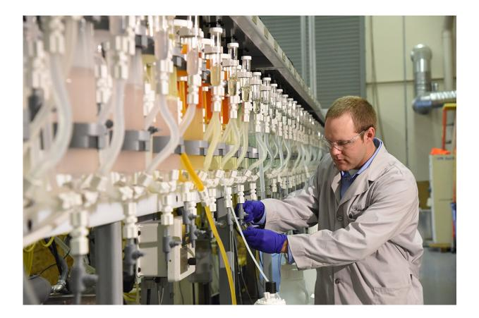
Kevin Lyon, an Idaho National Laboratory chemical engineer with expertise in applied solvent extraction, operates a counter-current solvent extraction system for testing and developing the process design for the separation technology. Credit: INL, U.S. Dept. of Energy
