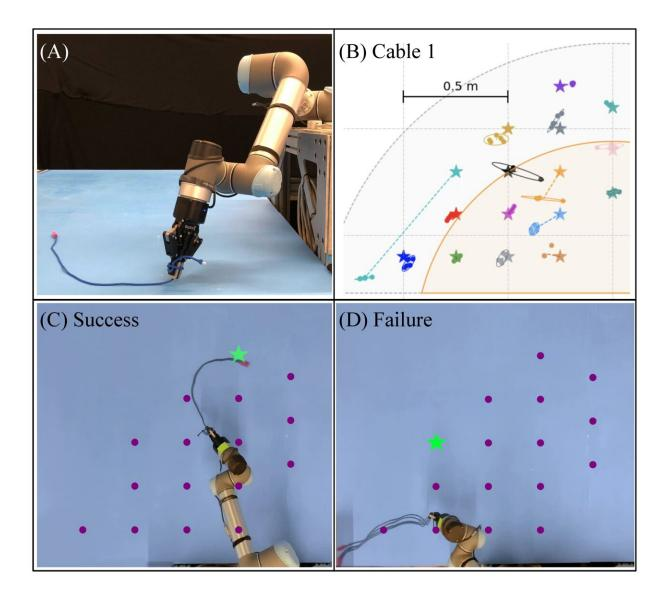
In Planar Robot Casting (PRC), a single planar motion of a robot wrist holding one end of a cable causes the other end of the cable to slide across the plane and
