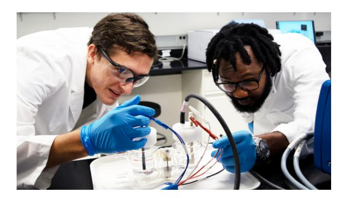
Denis Johnson and Dr. Abdoulaye Djire assemble the electrochemical cell used to perform the carbon dioxide reduction reaction experiments by connecting gas and electrical lines. Credit: Texas A&M Engineering
