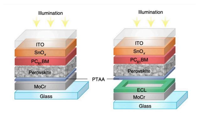
Figure showing the layout and structure of the device created by the researchers, with (left) and without (right) an edge cover layer (ECL). Credit: Breemen et al.
