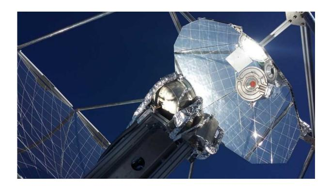
The sun-tracking parabolic reflector delivers concentrated sunlight to a solar reactor (seen via the secondary reflector) which converts water and  $CO_2$  extracted from the air into a syngas mixture, which in turn is further processed into drop-in fuels such as kerosene. Credit: ETH Zurich.
