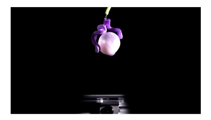
Princeton researchers have invented bubble casting, a new way to make soft robots using "fancy balloons" that change shape in predictable ways when inflated with air.
