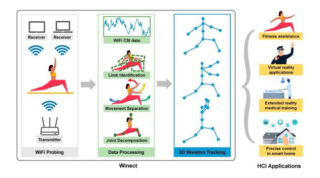
The Winect system transmits WiFi signals and analyzes their reflections off human body to generate dynamic 3D human skeletons. Credit: Ren & Yang.
