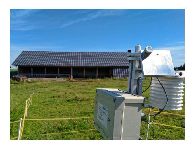
Analyses of the influence of aerosols on the yield of photovoltaic systems contribute to better utilisation of electricity grids and to making the energy transition more secure. A measurement campaign in Allgäu as part of the MetPVNet project provided important data for estimating the production of
