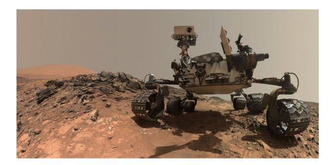
The Curiosity Mars rover, launched in November 2011, is powered by a nuclear battery that relies on thermoelectric materials to turn heat from radioactive decay into electricity. Credit: NASA/JPL-Caltech/MSSS, CC BY-NC
