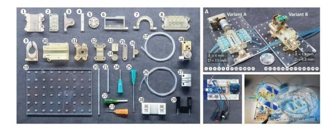
To make microfluidic pumps more accessible to the scientific community, SUTD researchers developed a highly-customisable, 3D-printed peristaltic pump kit, where users from around the world can download the design files, 3D-print and assemble their do-it-yourself peristaltic pump. Credit: SUTD
