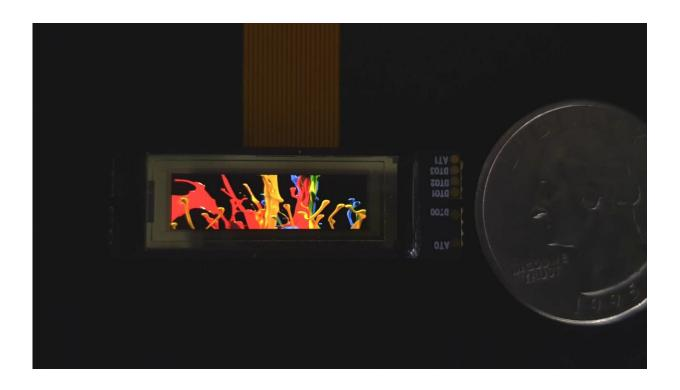
OLED micro-display panel with photoresist materials. Credit: Electronics and Telecommunications Research Institute(ETRI)
