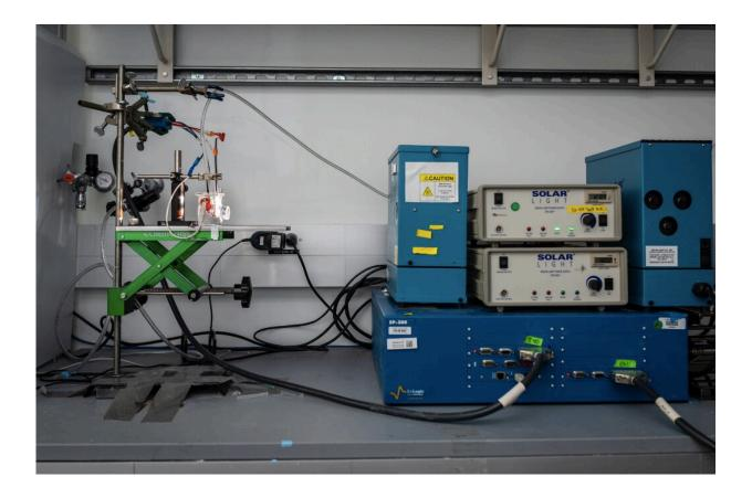
The researchers' artificial photosynthesis device converts CO2 emissions into ethylene and hydrogen fuels. Credit: Thor Swift/Berkeley Lab. © The Regents of the University of California, Lawrence Berkeley National Laboratory.
