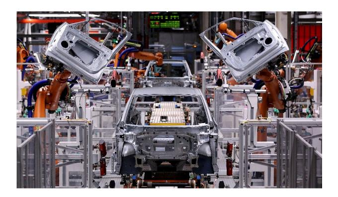
Robots mount doors on an ID.3 Volkswagen electric car. Germany's pivot to electric vehicles means carmakers are racing to retrain their workforces.
