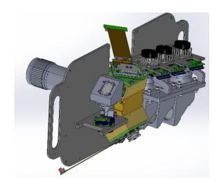
Figure 2. The developed projector has a unique optics engine (shown on the right) and two digital micromirror devices that enable it to project RGB and IR images with excellent alignment accuracy. Credit: Yoshihiro Watanabe from Tokyo Tech and the source and copyright of ITE and SID
