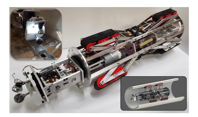
The pipe maintenance robot developed in the research. Credit: Kanazawa University
