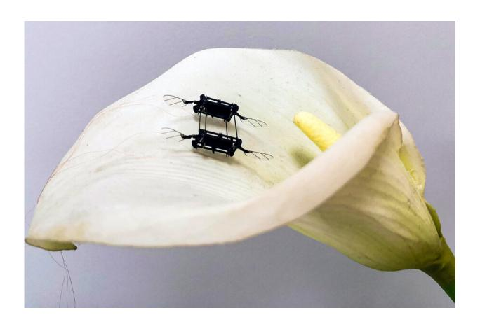
MIT researchers have pioneered a new fabrication technique that enables them to produce low-voltage, power-dense, high endurance soft actuators for an aerial microrobot. Credit: Massachusetts Institute of Technology
