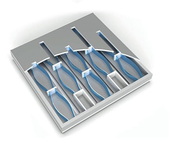
Lamella-like bending beams inside the MEMS microspeaker generate the sound. Credit: Arioso Systems GmbH
