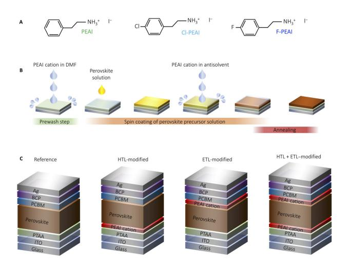
Fig. 1. Chemical structure of PEAI cations and schematics of the fabrication procedure and device architecture used in this work.(A) Chemical structure of PEAI, Cl-PEAI, and F-PEAI. (B) Schematic presentation of the fabrication procedure of the perovskite active layer. (C) Solar cell device structures with the different combinations of passivated interfaces. Credit: DOI: 10.1126/sciadv.abj7930
